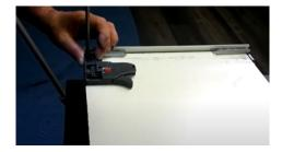
Now install the drawer clips into the pre-drilled holes in the front panel. Please note the orientation of the protruding portion of the clip – it should be towards the vertical center of the face:
