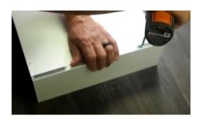
Next install the undermount drawer clips to the bottom using the bundled ½" screws. They should be aligned with the front edge of the bottom panel and right against the side panel:
