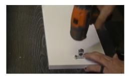
Then tighten the screw heads to firmly anchor the clip to the drawer base:
