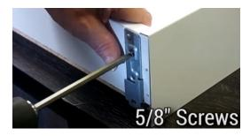
Turn the drawer box over and install 5/8" screws into each corner to secure the bottom panel to the sides:
