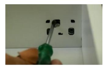
Next you will install your drawer slides, which will be fastened to the pre-drilled holes in the side panels using the included euro screws:
