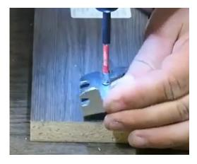
Next, install a system screw ("Euro Screw") on each side panel in the second hole from the bottom. Install the screw only halfway, so that the bracket on the toe kick latch onto it:
