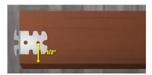
This will put the center bracket in alignment with the second hole from the bottom of your side panels.
